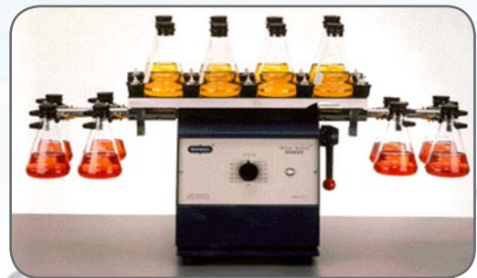
Dynamic Shake Flask Test (ASTM-E2149-01)
